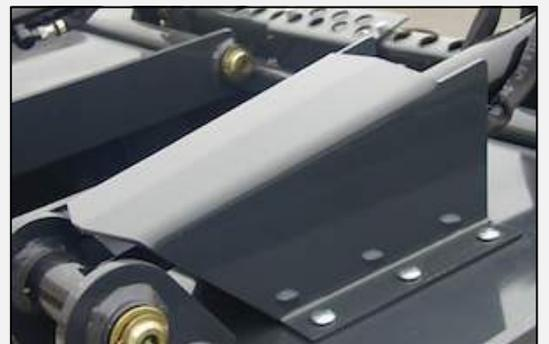
Guards protect cylinders from damage.
