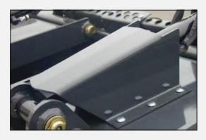
Guards protect cylinders from damage.
