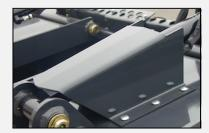
Guards protect cylinders from damage.
