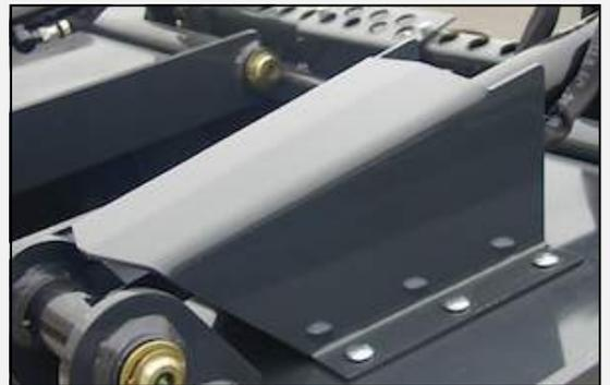
Guards protect cylinders from damage.
