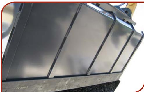
5 wear plates on underside of hopper bin
