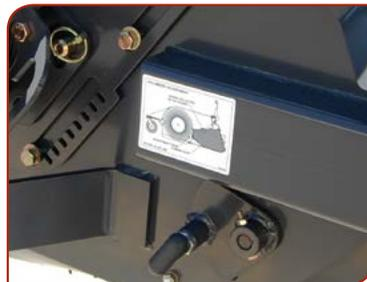
A simple tool-less adjustment knob allows you to accommodate brush wear and still maintain increased bucket capacity
