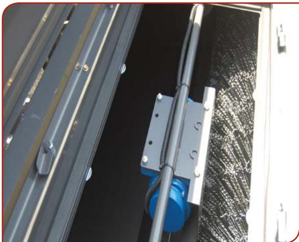
12 volt shaker dislodges loose debris from the filter media directly into the hopper
