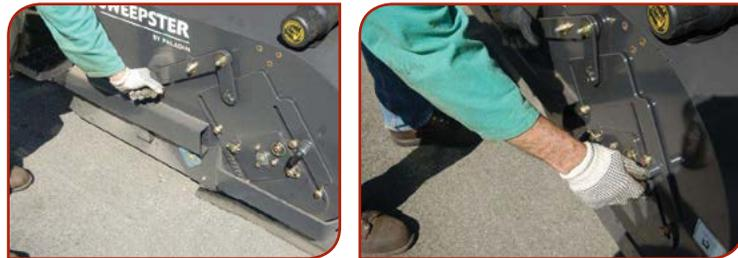
Hold onto brush adjustment lever. Grasp and pull T-handle quick pin out. Push lever to raise or lower brush head to desired height. Release T-handle quick pin ensuring notch is fully engaged.
