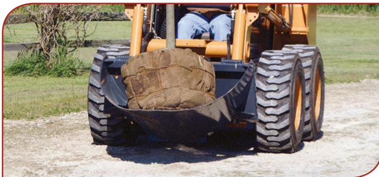
The **FFC Tree Scoop**, by Paladin, is designed for digging holes for tree planting or removal of trees. Very economical tree planter.
