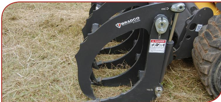
**Bradco Root Rake**, by Paladin, allows you to remove the toil and leave the soil at your job site with aggressive tine and grapple profiles that lock material in place and stabilize during transport.
