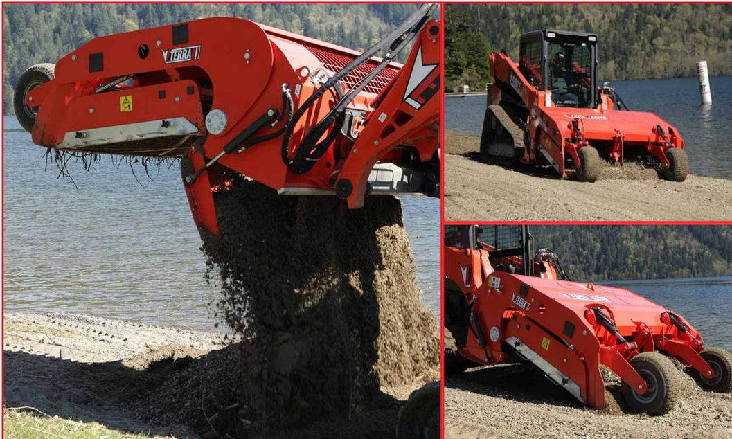
The **Eterra Beach Master** is an excellent tool for sifting through sand or light material and removing hazardous materials or just plain garbage. From cleaning up Hawaii's plastic beaches, to removing cigarette butts, glass, rocks and sticks from lake front properties; it's a safe bet to rely on the Beach Master.
